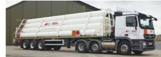
Hydrogen tube trailer, 350 kg capacity
